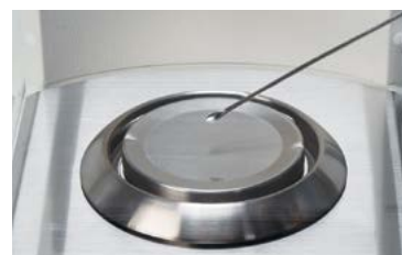
When the measurement spoon is electrically charged, and bringing it near the pan affects the numerical value
