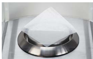
When the powdered medicine paper is electrically charged, and the numerical value is unstable
