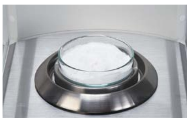
When the powder in the Petri dish is electrically charged, and the numerical value fluctuates
