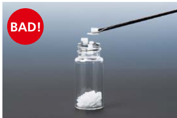
The sample is hard to handle because it adheres to the ampoule inlet and sides.
