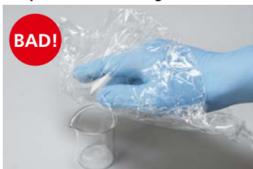
Plastic wrap adheres to rubber gloves, making it difficult to work with.
