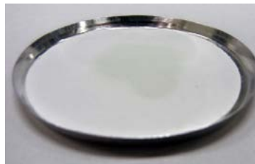
(Before measurement) 1 g of milk was dripped on to a fiberglass sheet for liquid measurement.
