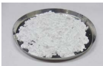
(Before measurement) The sample powder was spread evenly over the pan.
